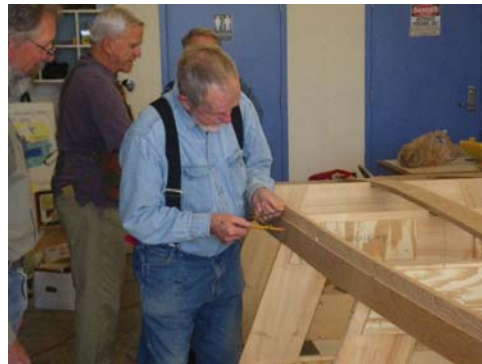
John spiling for the first plank
