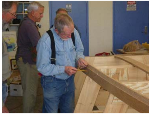
John spiling for the first plank
